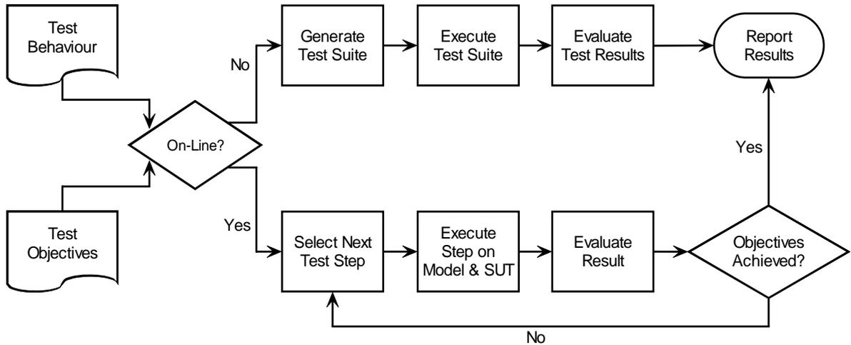
Figure 6: MBT Process – On-Line vs. Off-Line Testing [18]
