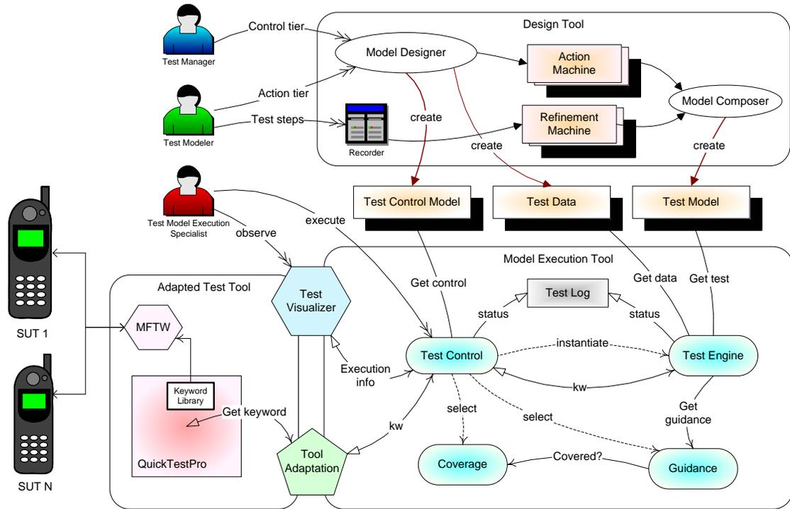
Figure 1: TEMA Tool Architecture Diagram [4]
