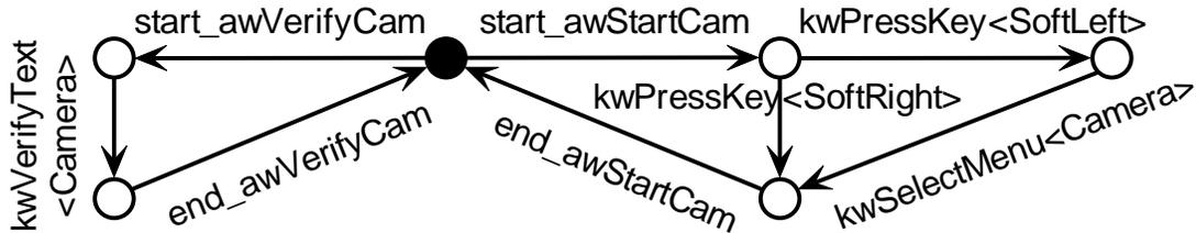
**Figure 4: Refinement Machine for Camera Action Machine [17]**
