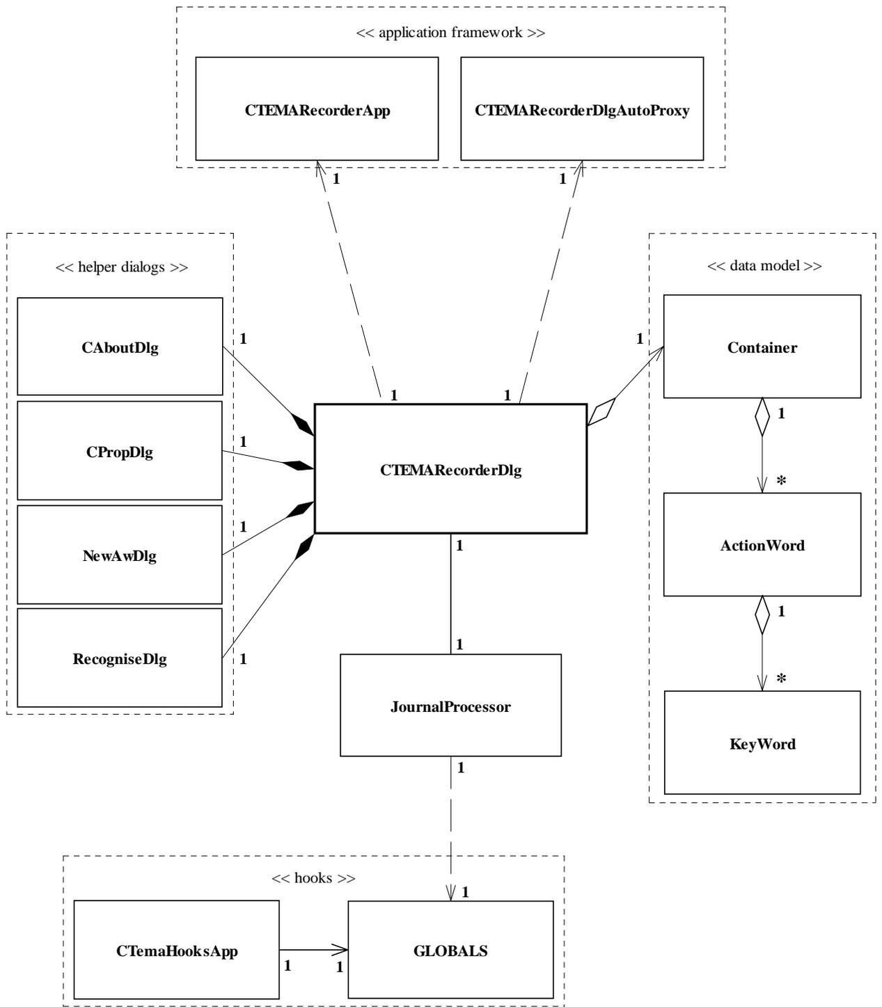
Figure 11: Recorder Class Diagram
