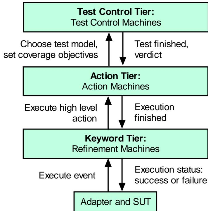
Figure 3: Three-Tier Test Model Architecture [17]
