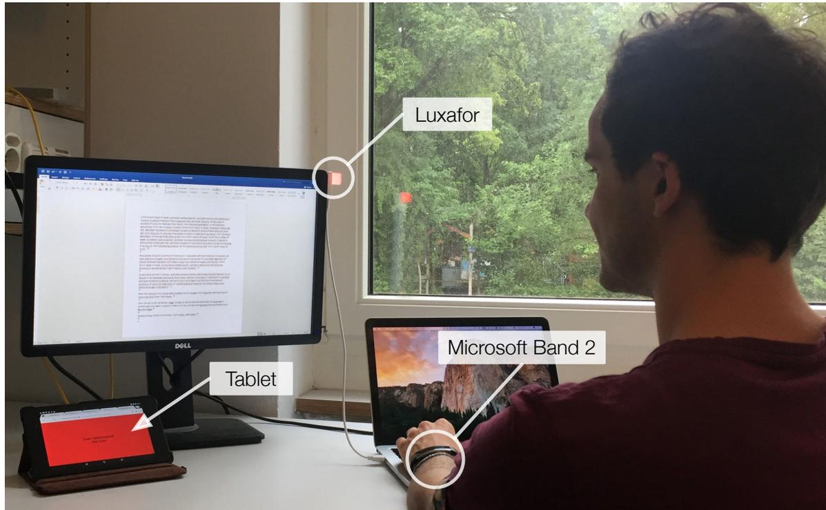
Fig. 6. The COLLINS system indicating that the office worker should not be interrupted.
