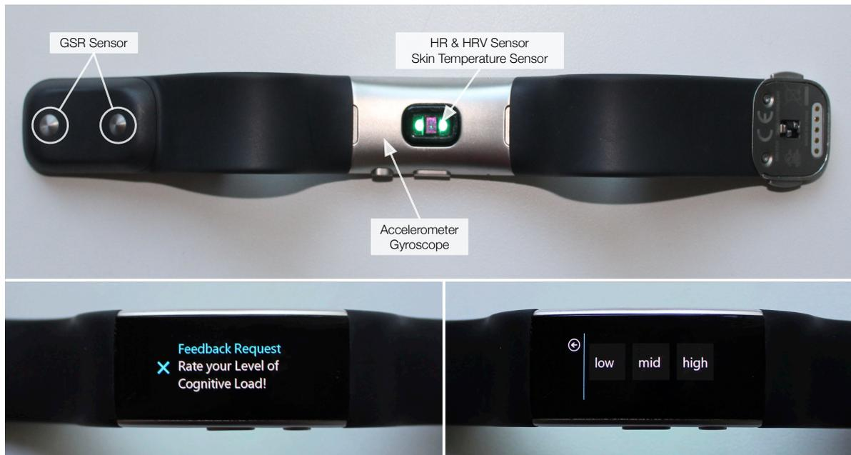
Fig. 3. Overview of the sensors of the Microsoft Band 2 (top). Screenshot of the notification of the feedback request (bottom left). The possible answers for the feedback request (bottom right).
